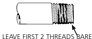
Figure 1. Pipe Compound Application
