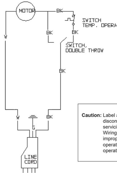
**Caution:** Label all wires prior to disconnection when servicing controls. Wiring errors can cause improper and dangerous operation. Verify proper operation after servicing.
