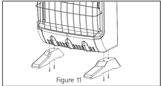
Note: Feet should have long end going out the front of heater, and the edge coinciding with side of heater. If feet overhang side of the heater, switch leg location.
